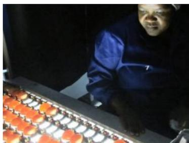
Less-than-perfect free-range eggs or those with hairline cracks checked on lights in a darkened cubicle join the liquid egg production line.
